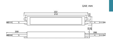
Model: JLI-60630KA Constant Current 10~60VDC 630mA 38W
